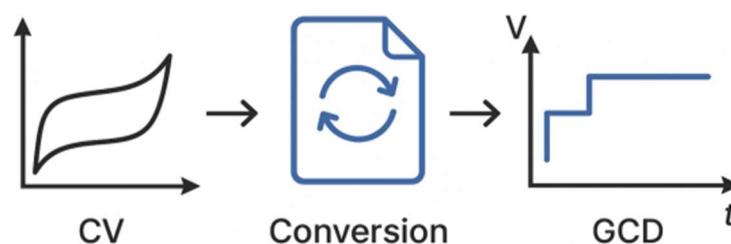
Figure 3: CV-to-GCD conversion for capacitance evaluation of CT complex.
