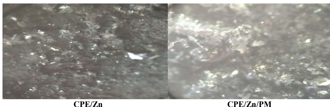
Figure 2: Optical surface image of CPE/Zn and CPE/Zn/PM.
