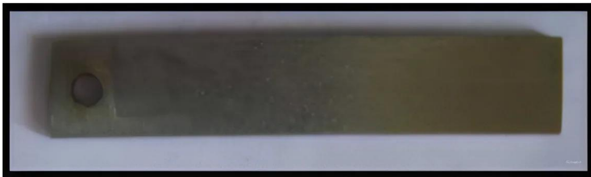
Figure 3: NiO thin film after 390 h salt spray test [54].
