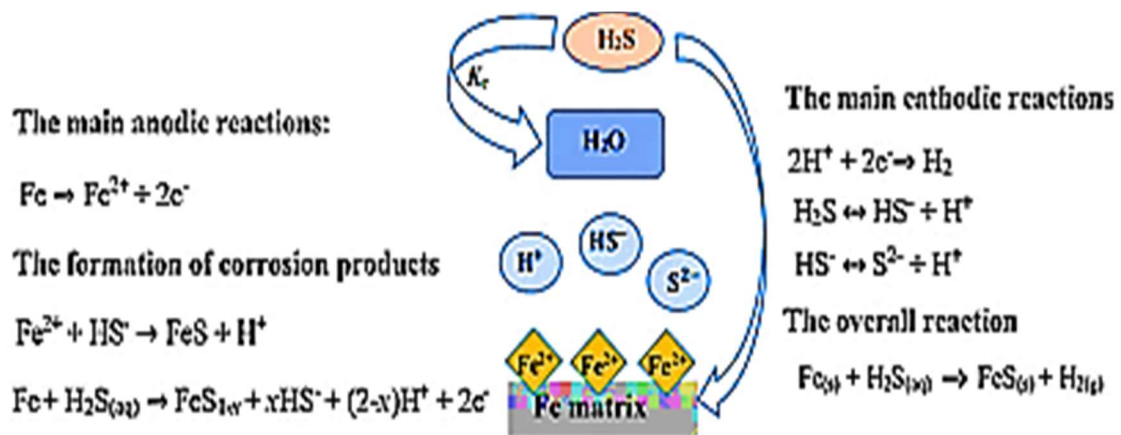
Figure 4: Schematic representation of steel corrosion reaction mechanism in an H 2 S environment.
