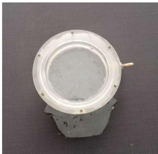
Figure 2: Transparent electrode with 87 mm diameter made of Hostaphan and filled with conductive liquid (1% CaCO 3 in a distilled H 2 O solution).
