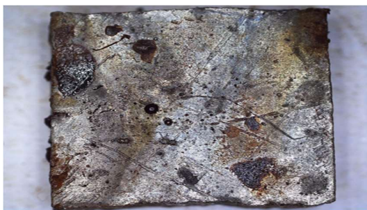
Figure 5: Effect of the \text{H}_2\text{SO}_4 solution on TS (without CP and after corrosion).
