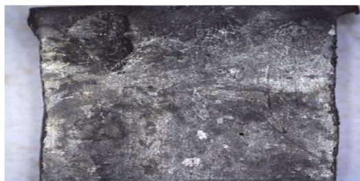
Figure 7: Effect of 5 mL CP on TS in a H 2 SO 4 solution (after corrosion).
