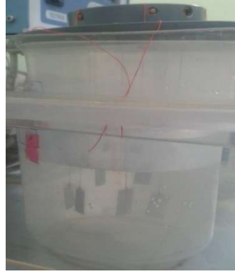
Figure 12: Al WL experiments in 500 mL of 3% NaCl.
