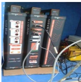
Figure 11: Origa Flex potentiostat.
