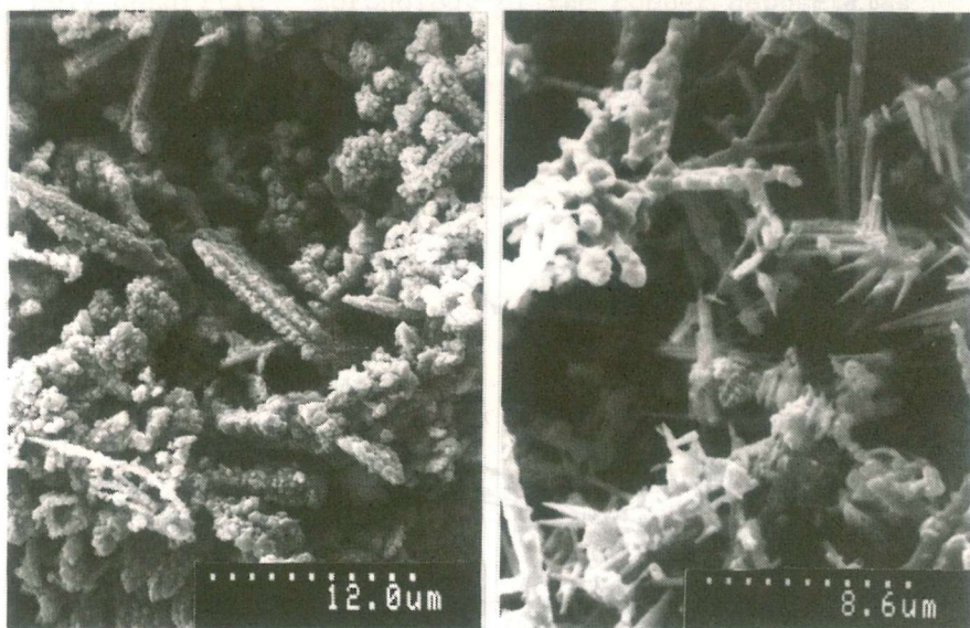
Fig 4 SEM's of copper deposits at pH 2.9 and 6.0
