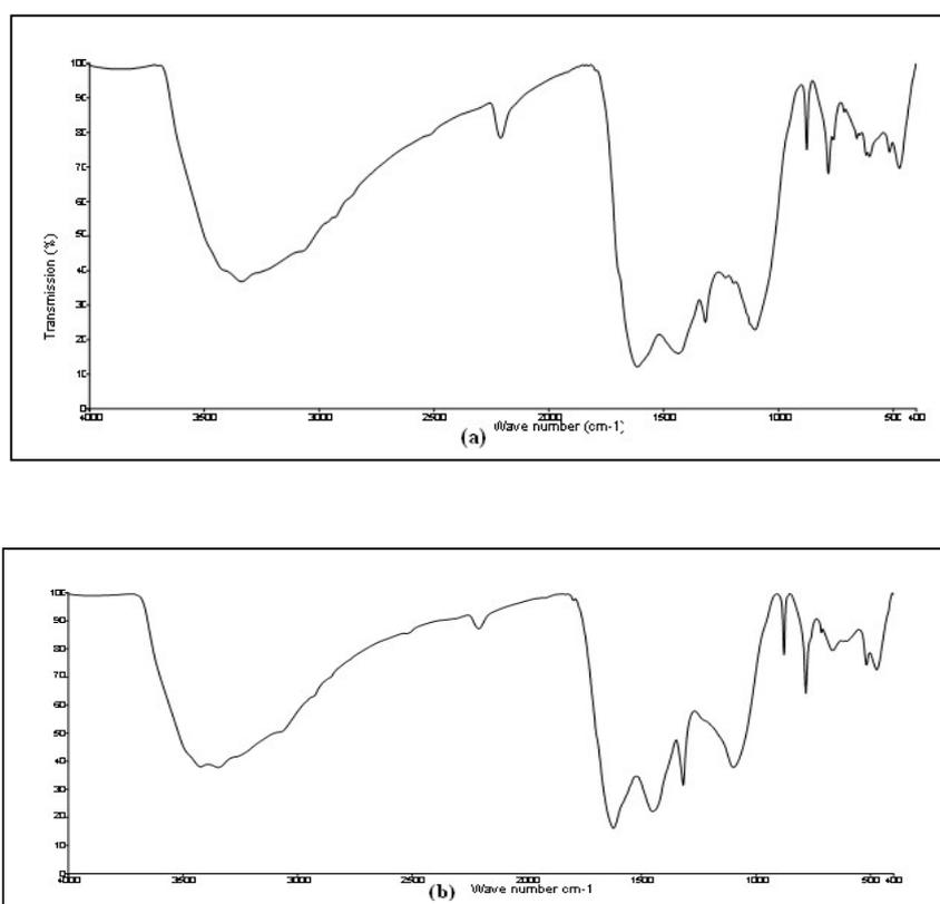
**Figure 4.** (a) FTIR spectrum of pure DBS; (b) FTIR spectrum of the film (Fe<sup>2+</sup>-DBS complex) formed on the MS surface after immersion in 0.25 mol/L H<sub>2</sub>SO<sub>4</sub> containing 100 mM DBS.
