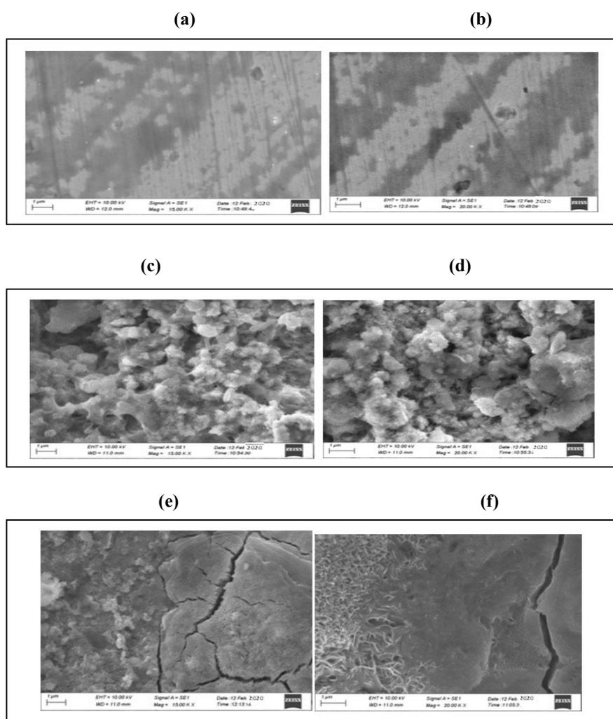
**Figure 5.** SEM analysis of MS: **(a)** magnification kX 15.00 (control); **(b)** magnification kX 20.00 (control); **(c)** in 0.25 mol/L  $\text{H}_2\text{SO}_4$ , magnification kX 15.00 **(d)** 0.25 mol/L  $\text{H}_2\text{SO}_4$ , magnif. kX 20.00; **(e)** 0.25 mol/L  $\text{H}_2\text{SO}_4$  + 100 mM DBS, magnif. kX 15.00 (control); and **(f)** 0.25 mol/L  $\text{H}_2\text{SO}_4$  + 100 mM DBS, magnif. kX 20.00kX 20.00 (control).
