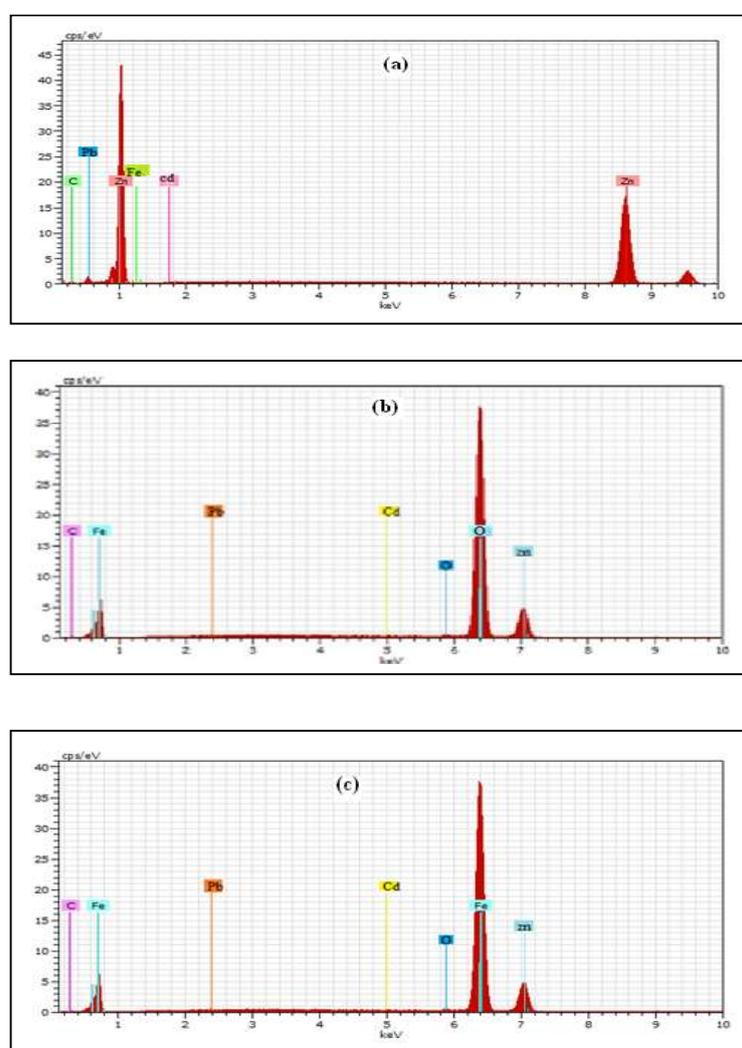
**Figure 6.** EDAX spectrum of: (a) MS specimen (control); (b) MS after immersion in 0.25 mol/L H<sub>2</sub>SO<sub>4</sub>; c) MS specimen after immersion in 0.25 mol/L H<sub>2</sub>SO<sub>4</sub> + 100 mM DBS.
