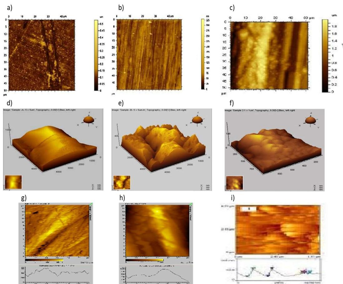
**Figure 7.** AFM images of MS at different conditions: polished surface (control) – **a)** 2D, **d)** 3D and **g)** cross-sectional profiles; immersed in 0.25 mol/L H<sub>2</sub>SO<sub>4</sub> – **b)** 2D, **e)** 3D and **h)** cross-sectional profiles; and immersed in 0.25 mol/L H<sub>2</sub>SO<sub>4</sub> + 100 mM DBS – **c)**: 2D, **f)** 3D and **i)** cross-sectional profiles.
