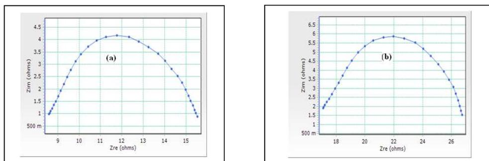
**Figure 2.** a. ACIS of MS immersed in 0.25 mol/L H<sub>2</sub>SO<sub>4</sub>, without DBS; b. ACIS of MS immersed in 0.25 mol/L H<sub>2</sub>SO<sub>4</sub>, without DBS and with it.
