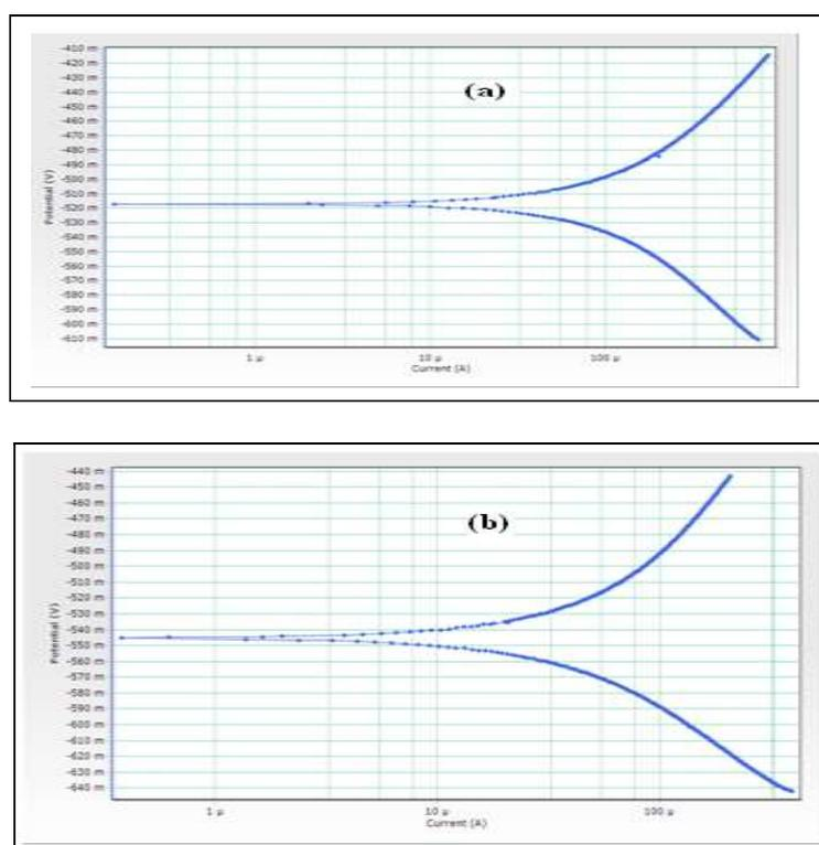
**Figure 1.** PDP curves of MS immersed in test solutions: (a) 0.25 mol/L H<sub>2</sub>SO<sub>4</sub> (blank); (b) 0.25 mol/L H<sub>2</sub>SO<sub>4</sub> + 100 mM DBS.
