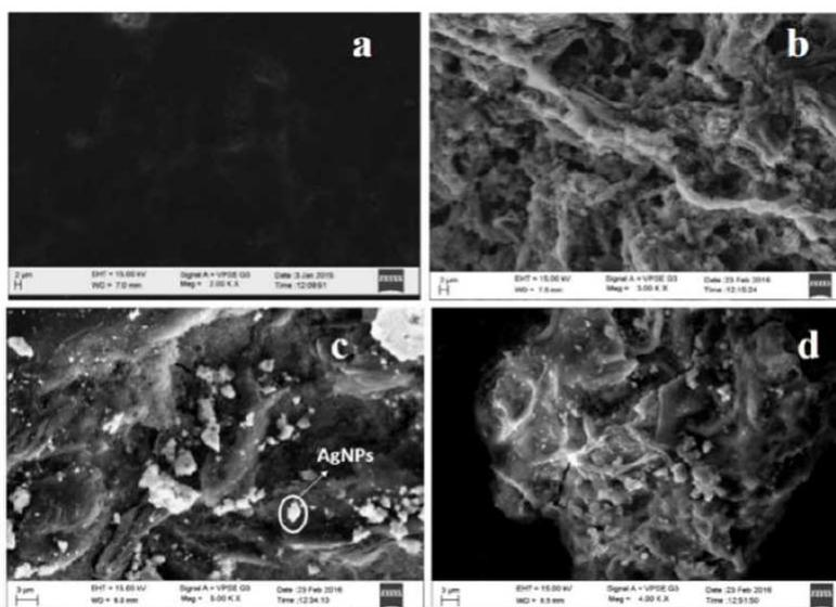
**Figure 2.** SEM images of a) Bare Gr, b) Gr/PPy, c) Gr/PPy/AgNPs and d) Gr/PPy/AgNPs/PPO electrodes surface.
