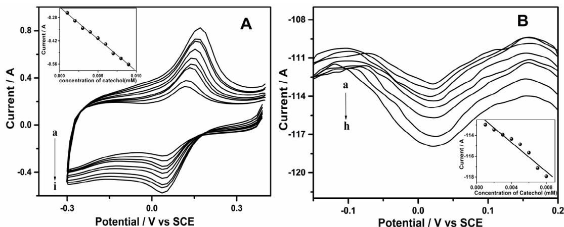
**Figure 4.** (A) Cyclic voltammograms of the Gr/PPy/AgNPs/PPO electrode with the successive addition of 0.001-0.009 mM catechol in 0.1 M PBS at pH 7. The inset shows the calibration plot of current vs. catechol concentration. (B) DPVs of the Gr/PPy/AgNPs/PPO electrode at varying catechol concentrations (0.001 – 0.008 mM) in a 0.1 M PBS solution. The inset plot shows the calibration plot of the peak current versus catechol concentration.
