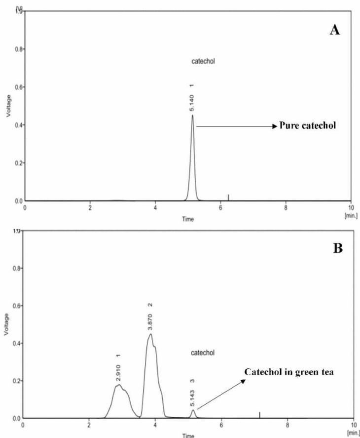
**Figure 7.** (A) HPLC chromatograms of standard catechol. (B) Green tea sample containing catechol. Catechol retention time: 5.14 min.
