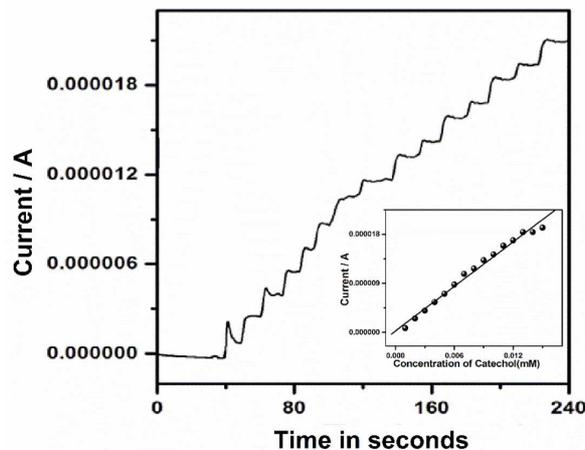
**Figure 6.** Chrono amperometric response of the Gr/PPy/AgNPs/PPO electrode in different catechol concentrations, at an applied potential of +0.025 V. The inset plot shows the calibration curve of the response current vs. catechol concentration.
