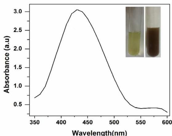
**Figure 1.** UV-vis spectra of biosynthesized AgNPs.
