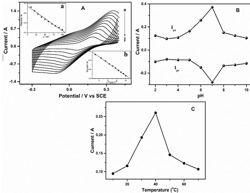
**Figure 5.** (A) Cyclic voltammograms of Gr/PPy/AgNPs/PPO in 0.1 M PBS at pH 7 containing 0.004 mM catechol at different scan rates (10-100 mVs<sup>-1</sup>); inset plots a) peak current vs. scan rate, b) peak current vs. square root of scan rate. (B) Effect of varying pH (from 2 to 10) on the peak current. (C) Effect of varying temperature (from 10 to 70 °C) on the peak current.
