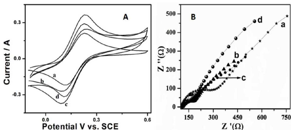
**Figure 3.** (A) CVs of a 5 mM  $[\text{Fe}(\text{CN})_6]^{-3/4}$  solution obtained for a) bare Gr, b) Gr/PPy, c) Gr/PPy/AgNPs and d) Gr/PPy/AgNPs/PPO. (B) Impedance spectra of a) bare Gr, b) Gr/PPy, c) Gr/PPy/AgNPs and d) Gr/PPy/AgNPs/PPO.
