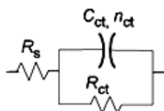
Figure 9. Equivalent circuit used to model impedance data in 1.0 M HCl solutions in the presence of different concentrations of M-Qn.
