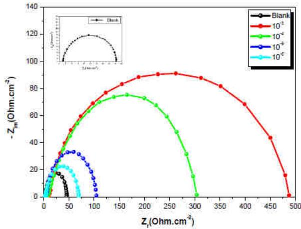
**Figure 4.** Nyquist diagrams for copper electrode in (2 M H<sub>3</sub>PO<sub>4</sub>+ 0.3 M NaCl) containing different concentrations of PPB, after 30min of immersion at E<sub>corr</sub>.
