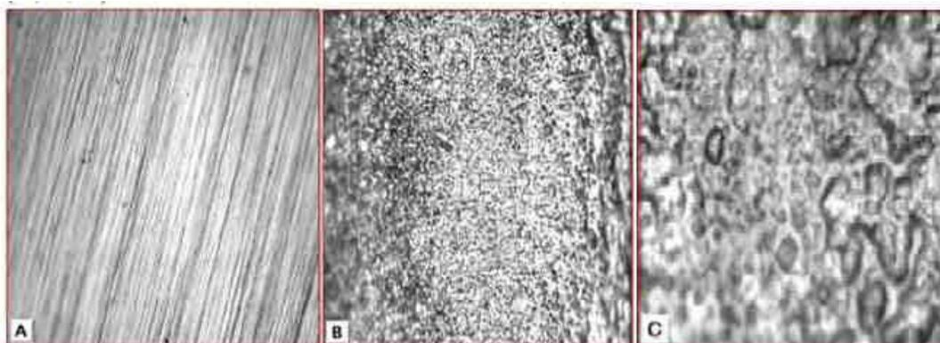
**Figure 13.** OM (x200) of copper (a) before immersion (b) after 6h of immersion in  $\text{H}_3\text{PO}_4$  2 M + 0.3 M NaCl (C) after 6h of immersion in 2 M  $\text{H}_3\text{PO}_4$  + 0.3 M NaCl +  $10^{-3}$  M (PPB) at 298 K.
