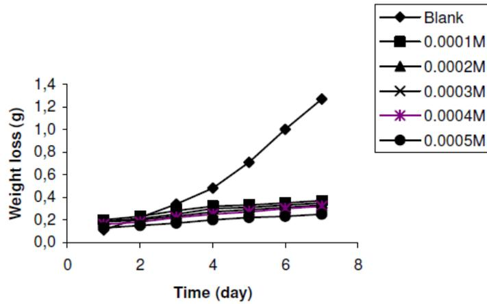
**Figure 2a.** Variation of weight loss with time for the corrosion of zinc in 0.01 M tetraoxosulphate (VI) acid containing various concentrations of lincomycin at 303 K.
