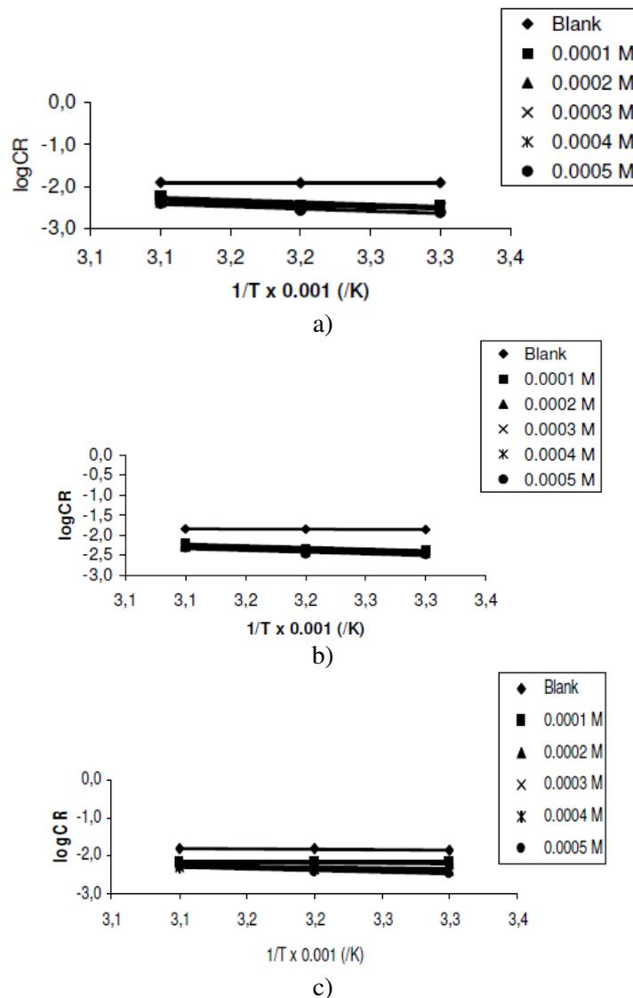
**Figure 4.** Variation of  $\log(CR/T)$  with  $1/T$  for the inhibition of the corrosion of Zn in (a) 0.01 M, (b) 0.02 M and (c) 0.03 M tetraoxosulphate(VI) acid by lincomycin.
