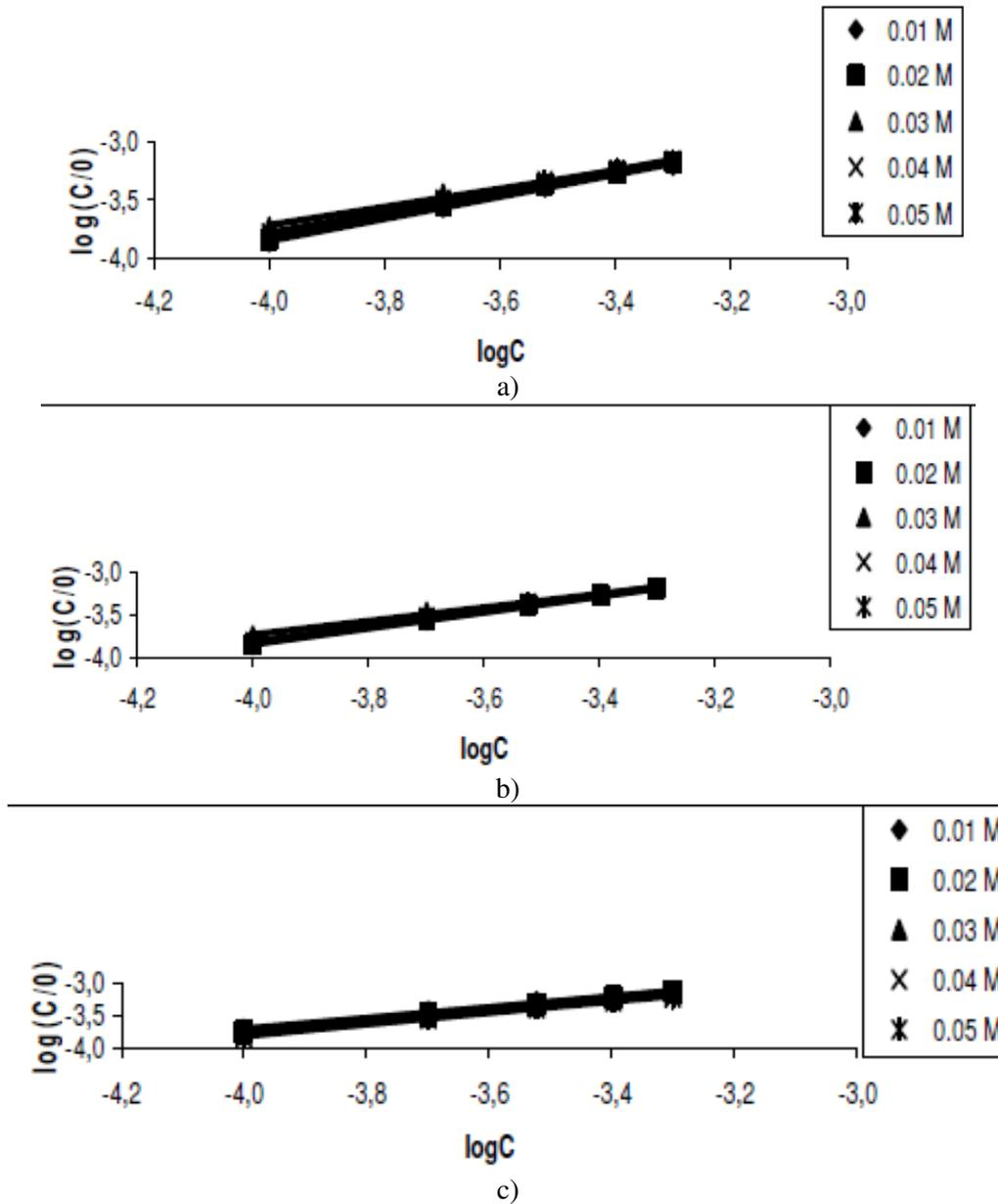
**Figure 5.** Langmuir isotherm for the adsorption of lincomycin on zinc surface in various concentrations of tetraoxosulphate (VI) acid at (a) 303 K, (b) 313 K and (c) 323 K.
