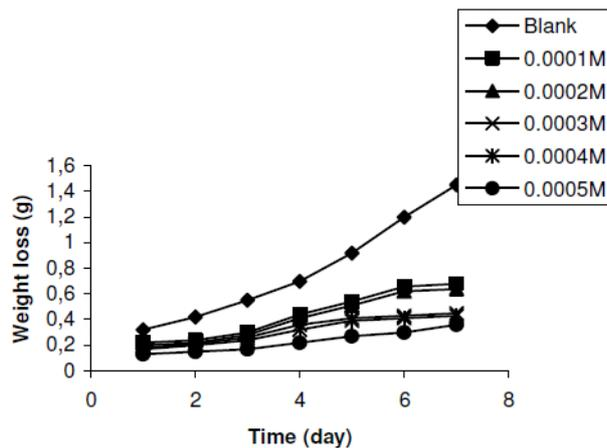
**Figure 2c.** Variation of weight loss with time for the corrosion of zinc in 0.03 M tetraoxosulphate (VI) acid containing various concentrations of lincomycin at 303 K.
