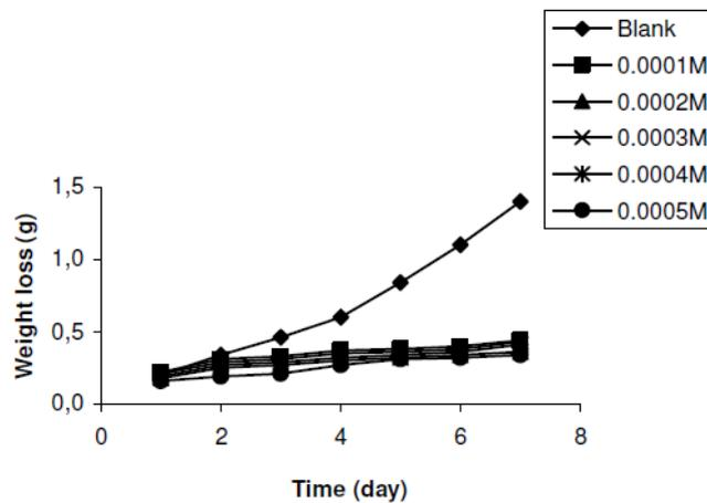
**Figure 2b.** Variation of weight loss with time for the corrosion of zinc in 0.02 M tetraoxosulphate (VI) acid containing various concentrations of lincomycin at 303 K.
