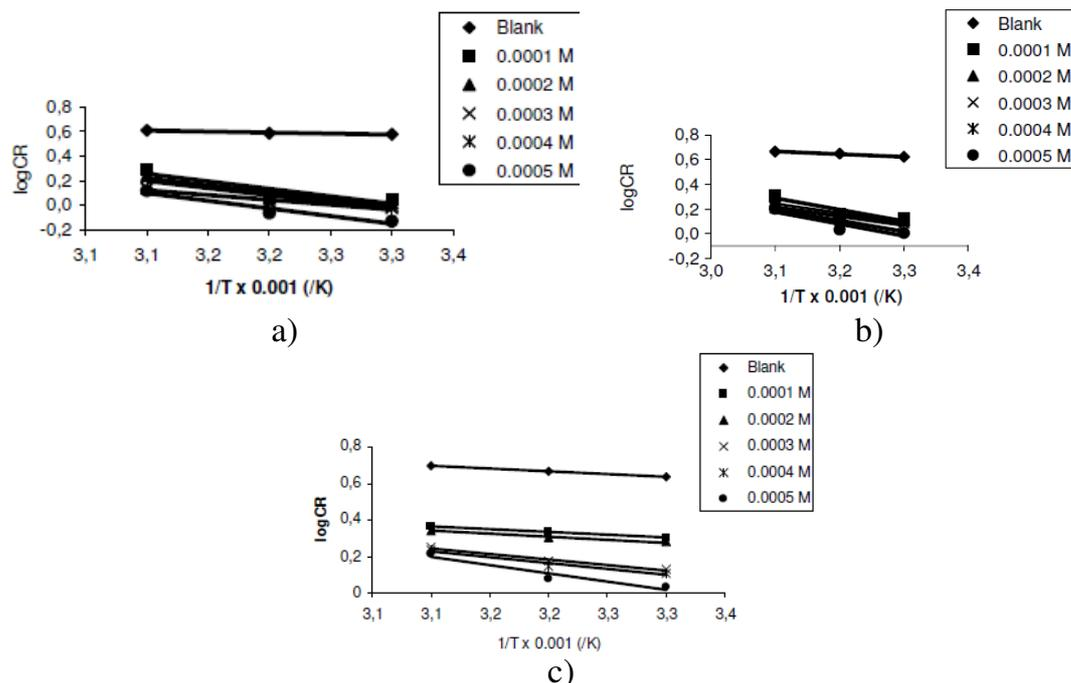
**Figure 3.** Variation of log(CR) with 1/T for the inhibition of the corrosion of Zn in (a) 0.01 M, (b) 0.02 M and (c) 0.03 M tetraoxosulphate(VI) acid by lincomycin.
