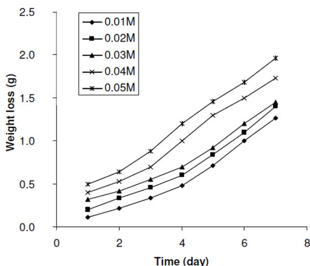
**Figure 1.** Variation of weight loss of Zn in various concentrations of tetraoxosulphate (VI) acid at 303 K.
