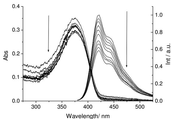
**Figure 3.** Change in absorption and emission of CCP-S with [dsDNA] increasing from 0 to  $12.4 \times 10^{-8}$  M base pairs.
