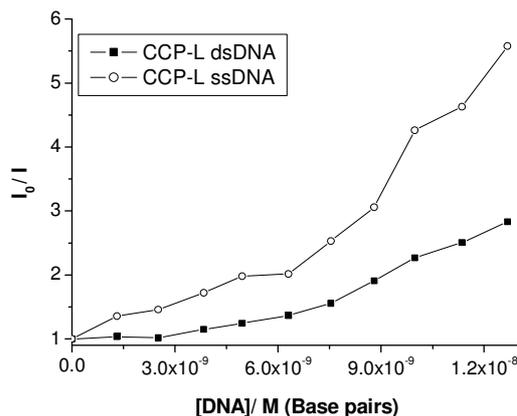
**Figure 4.** Stern-Volmer plots for quenching of CCP-L fluorescence by DNA.
