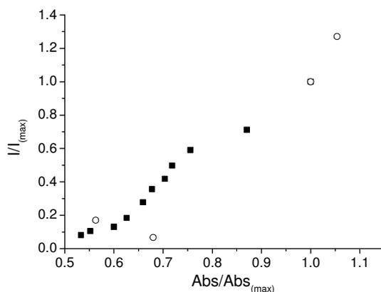
**Figure 5.** Ratio of emission against ratio of absorbance for CCP-L for changes in solvent composition (open circles ) and quencher concentration (filled squares).
