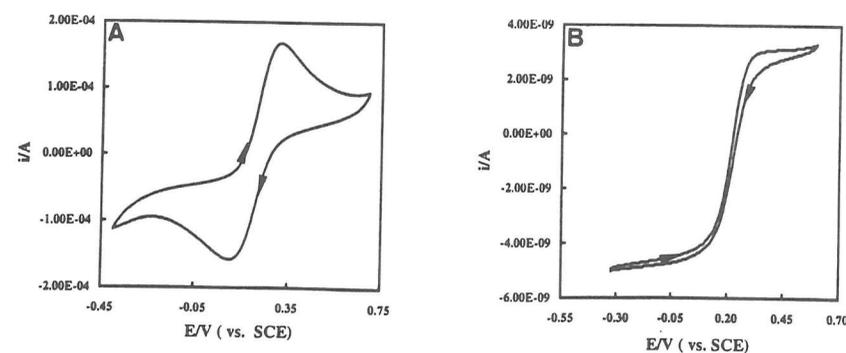
**Figure 3-** Cyclic voltammograms of Fe<sup>3+</sup> in  $\alpha$ -MEM Supply: (A) 200  $\mu$ g/mL of Fe<sup>3+</sup> using a conventional Au electrode at  $v=10$  mV/s; (B) 150  $\mu$ g/mL of Fe<sup>3+</sup> using a Au microelectrode at  $v=50$  mV/s.
