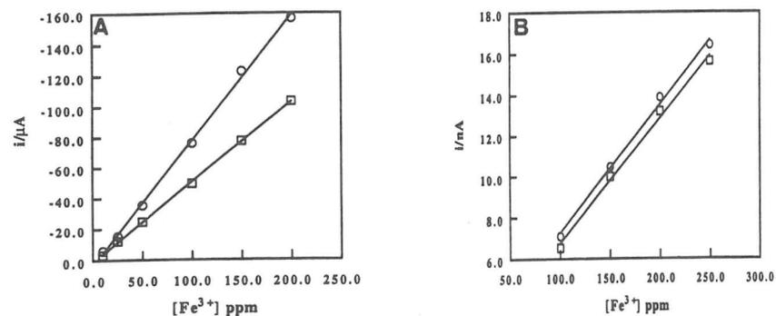
**Figure 4-** Calibration curves of  $\text{Fe}^{3+}$  in  $\alpha$ -MEM Supply obtained with: (A) a conventional Au electrode at ( $\square$ )  $v=5$  mV/s and ( $\circ$ )  $v=10$  mV/s; (B) a Au microelectrode at ( $\square$ )  $v=75$  mV/s and ( $\circ$ )  $v=150$  mV/s.
