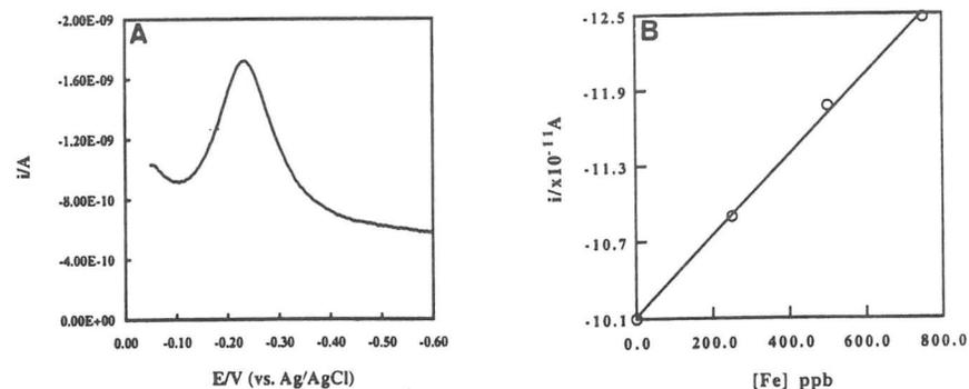
**Figure 5-** Determination of dissolved Fe in osteoblast-like cell cultures medium: (A) cathodic stripping voltammogram; (B) calibration graph obtained by additions of a standard solution of iron to the sample.
