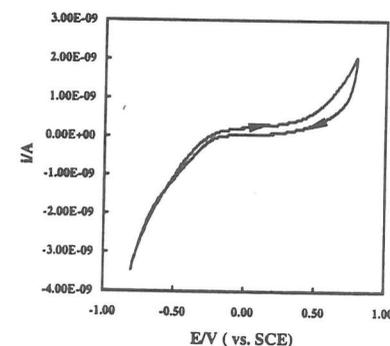
**Figure 2-** Typical cyclic voltammogram of osteoblast-like cell cultures medium obtained with a 25  $\mu$ m Au microelectrode at a scan rate of 100 mV/s.
