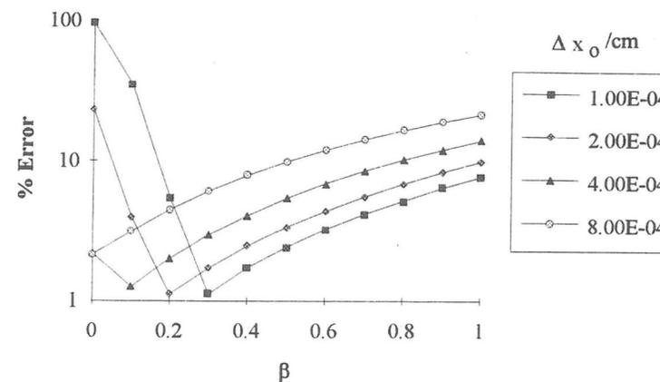
Figure 4 - Evolution of the average error (in percentage) as a function of  $\beta$ , for various values of  $\Delta x_0$  (cm).
